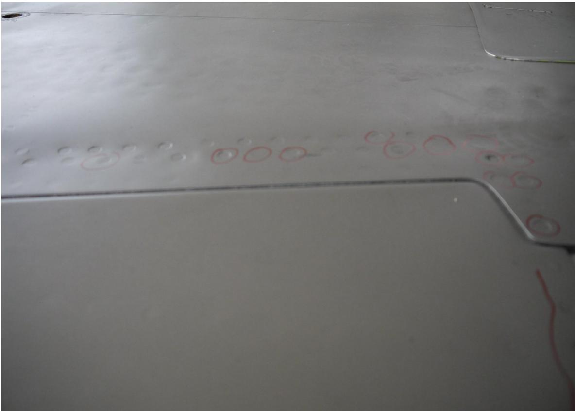
The red circles indicate the damaged rivet heads in the main spar area.
