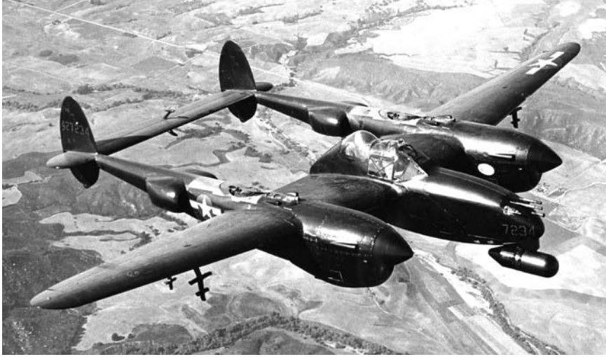
The P-38M night fighter was ready for combat. Notice the antennas under both the left and right wings, and the bomb-shaped nose pod.
