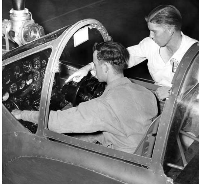
P-38 cockpits had plenty of room and almost twice as many instruments as other fighters.
