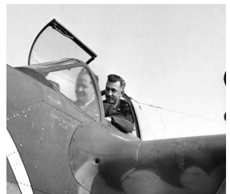
Lockheed's P-38 was the first fighter to use the two-seat system. Other first-line fighter training systems later adopted it. Test pilot Jimmie Mattern (front) and Army Air Forces ace Maj. Clarence Shoop show the tight fit of the piggyback trainer.
