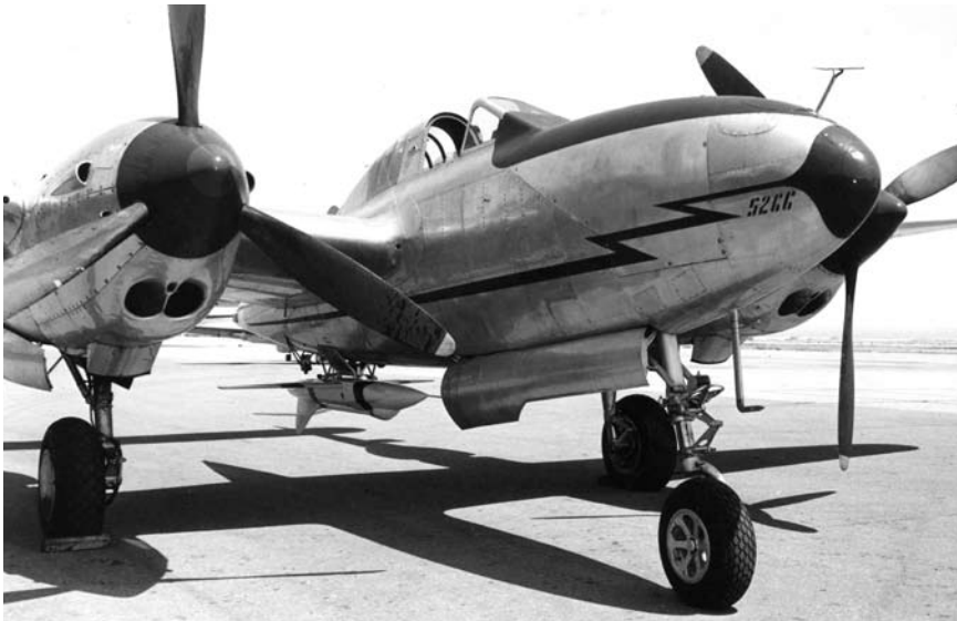
A post-World War II Lightning with a scale-model F-80 jet mounted on its underside for early tests.
