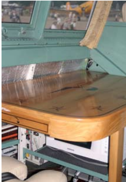
Navigator's table of inlaid wood reflects the craftsmanship of the restoration. Note microwave below chart table.
