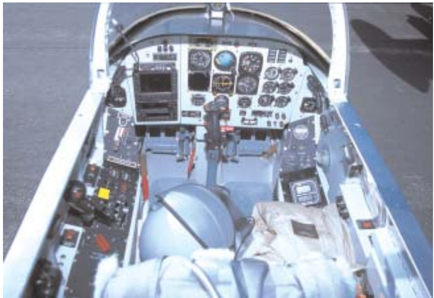
The modernized instrument package and fire warning system required more than 7,000 feet of wire.
