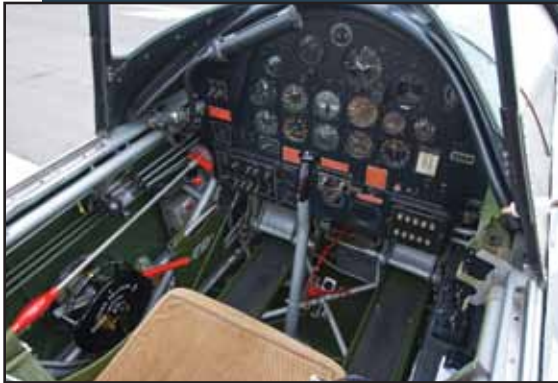
Cockpit details: note large fluorescent lamp on flexible arm for panel illumination at night.
