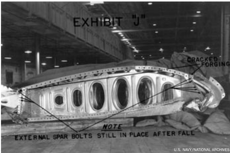
After recovery from in front of the Kingsley St. home, the left outer wing panel was thoroughly examined. It was quickly determined that workers failed to connect the panel by omitting 98 bolts. Only the four spar attach bolts were installed, having failed shortly after takeoff.
