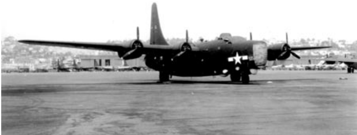
A factory-fresh PB4Y-2 is seen on the ramp at Lindbergh Field, San Diego. Notice that the aircraft has been fitted with an aerodynamic covering over the location where the nose turret will be installed. This is the configuration of BuNo 59554 when it took off on November 22, 1944.
