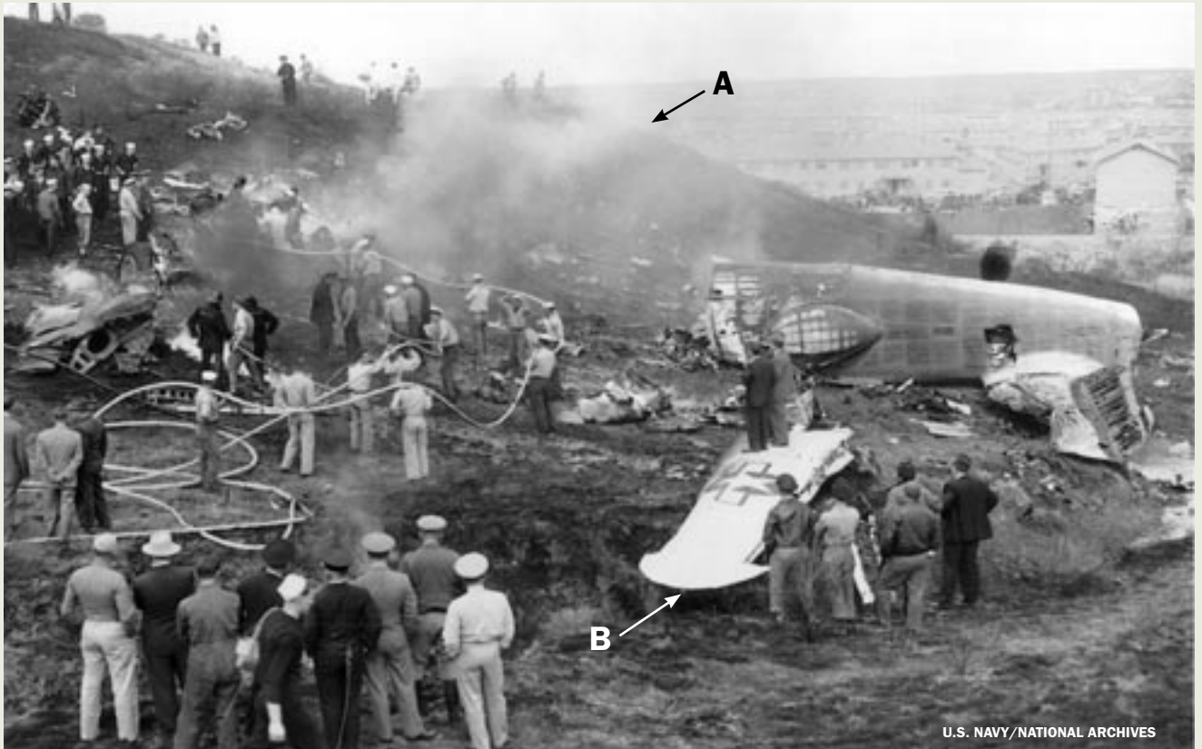
Above: At the impact site of BuNo 59554, Navy crews worked to rescue any possible survivors. Notice the hole chopped into the rear fuselage near the horizontal stabilizer. 'A' denotes the unusual shoulder of the hill, and 'B' shows the starboard outer wing panel lying across a drainage ditch.
