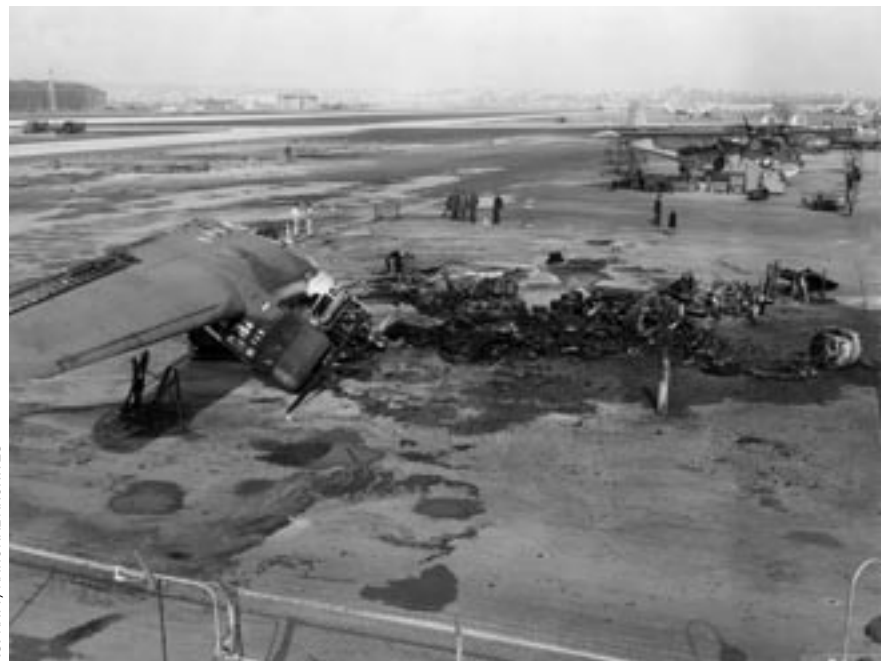
When an unqualified mechanic attempted to remove a battery solenoid, he broke a hydraulic line. The subsequent fluid spill ignited with the results shown here. BuNo 59350, the first production PB4Y-2, was completely destroyed.
