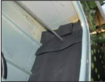
Dennis Savarese's FOD Prevention Cover (looking back and up into the tail).
