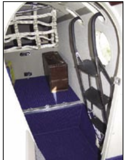
Unique ladder stowage installation in Dewey's Ride.
