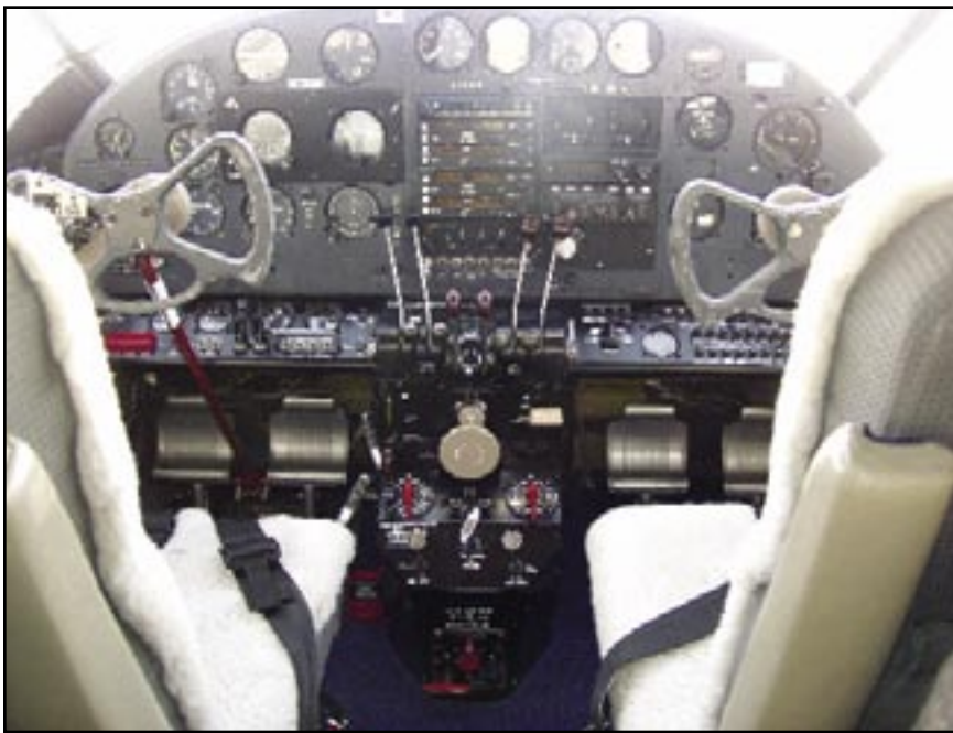
Refurbished panel for dual pilot operations.
