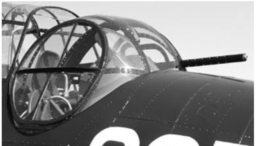
The Grumman 150CE turret's single .50-cal. machine gun was off-set to the left of the turret, or to the right of the aircraft centerline when facing aft. The turret used the Mk. IX "mail box" reflector gunsight.
