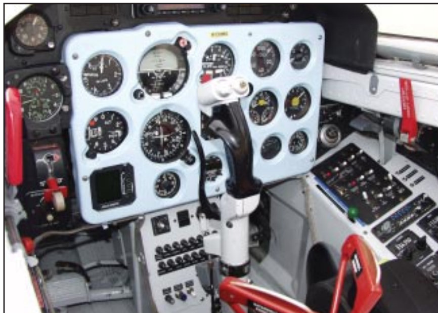
Splashes of red in the Pig's cockpit denote devices used to pop the canopy and engage the hot ejection seat in an emergency.
