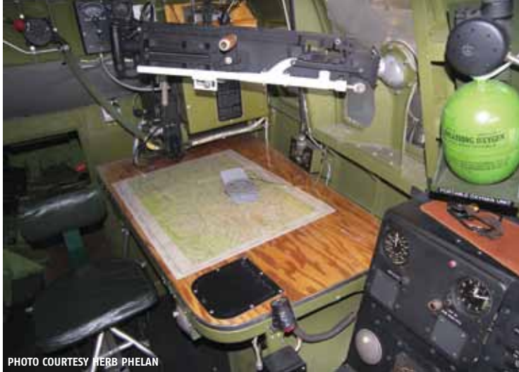
The new navigator's table on port side with gun, oxygen tank, and other equipment.
